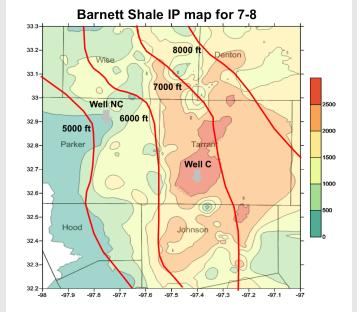
Exhibit 11: IP & depth map for core of Barnett shale play, with dummy wells (Source: HPDI and Kimmeridge Energy)
