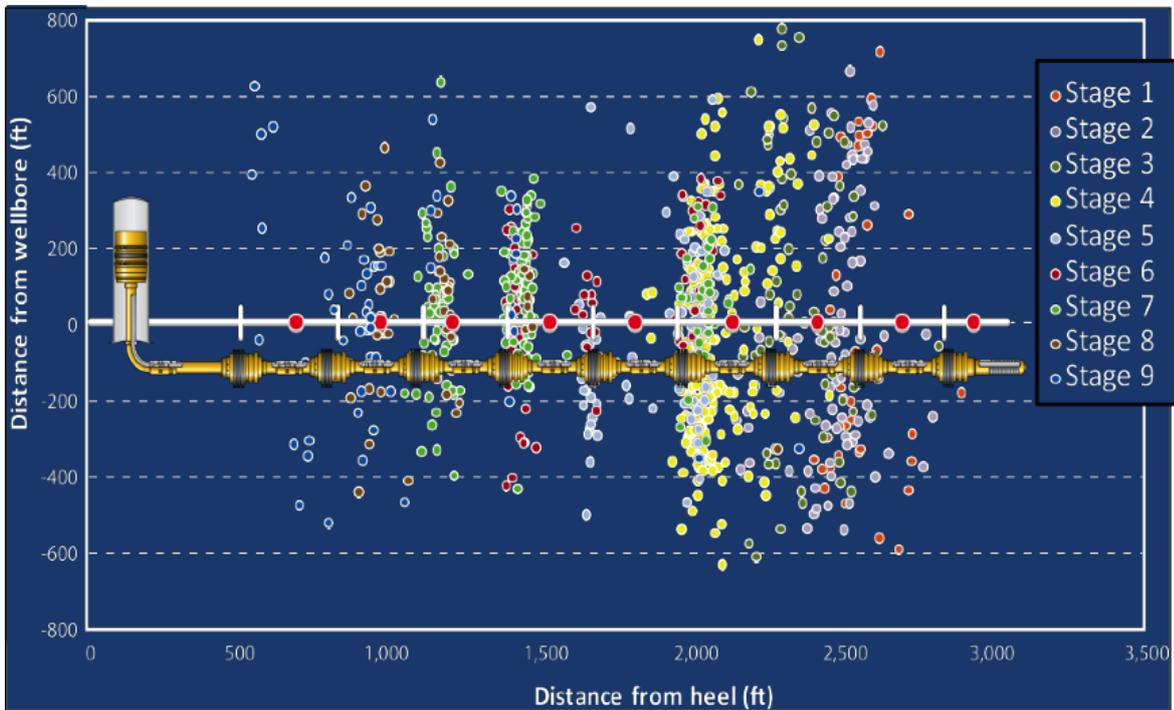
Exhibit 4: The micro seismic response of different frac stages with each bubble associated with the propagation of an individual fracture. (Source: Baker Hughes)
