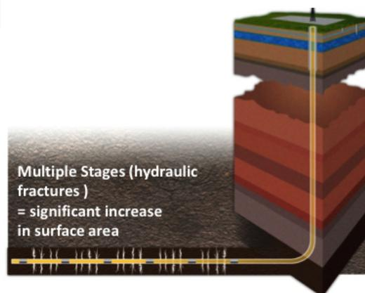
Exhibit 1: The impact of hydraulic fracturing on the surface area exposed to the wellbore. (Source: Baker Hughes)
